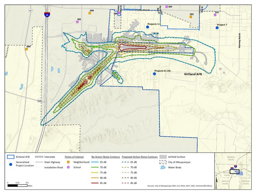
Figure 4-1 Noise Exposure: Proposed Action vs. No Action DNL Contours
