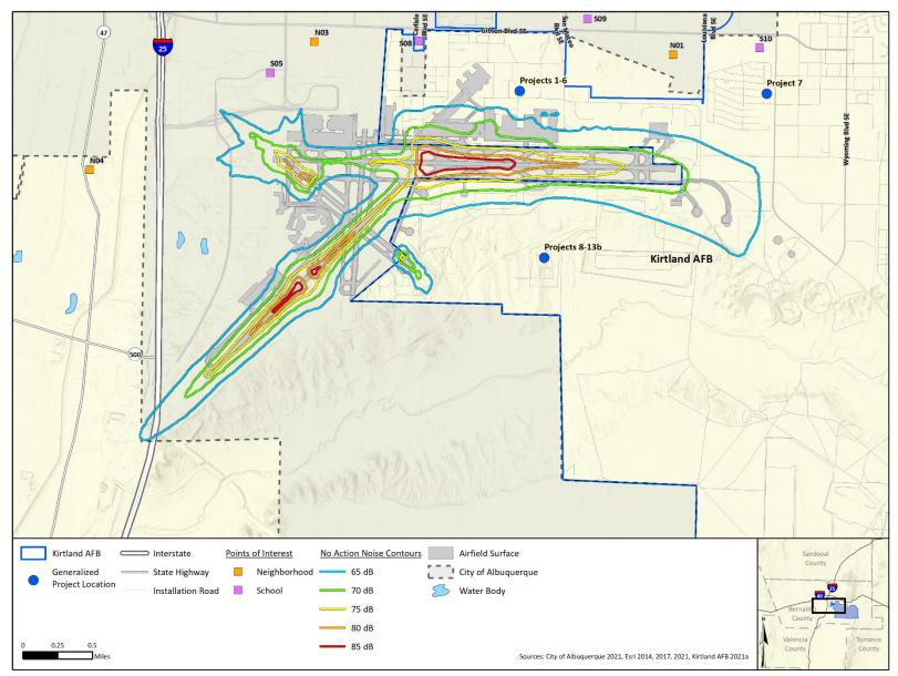
Figure 3-1 Noise Exposure: No Action Alternative DNL Contours
