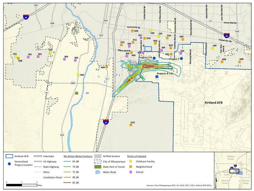
Figure 3-2 Noise Exposure: No Action Alternative DNL Contours, showing POIs
